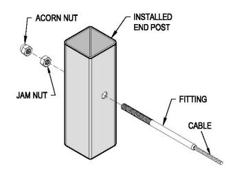
**DO NOT CRIMP.** Pull the cable taut, making sure it remains 'bottomed out' inside the fitting. Measure from the outside of the post to the near side of the jam nut. Trim this amount from the cable and attach the fitting as you did in Step A. (Note: you will have to pull the cable out of the last post to do this).
