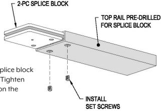
**NOTE**: Straight lengths of top rail will follow the pitch of the mounting surface, so leveling them is unnecessary.
