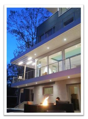
contrast to glass railings, which would have been the only other alternative for a transparent, modern railing, a cable railing system requires a lot less maintenance and cleaning to stay attractive, it visually disappears since it does not show reflections, it is light-weight and eventually fully recyclable – really the only choice for this project."
